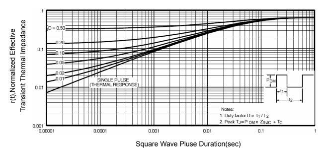
Figure 11 Normalized Maximum Transient Thermal Impedance
