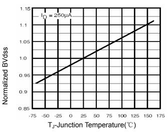
Figure 9 BV<sub>DSS</sub> vs Junction Temperature
