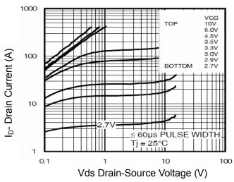
**Figure 1 Output Characteristics**
