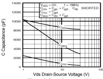
Figure 7 Capacitance vs Vds
