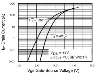
**Figure 2 Transfer Characteristics**
