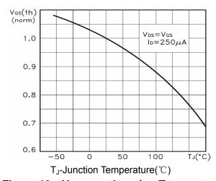
Figure 10 V<sub>GS(th)</sub> vs Junction Temperatur
